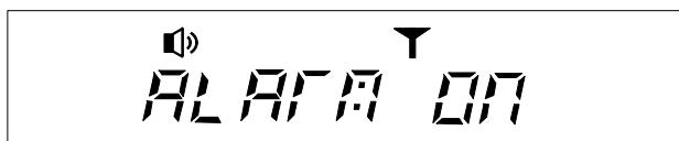
③ Press the function button, pager is in alarm setting mode.. The hour digits blink.
