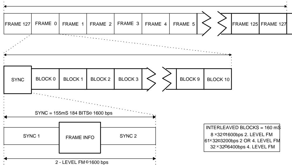
The Sync 2 portion of the frame is designed to provide synchronization at the frame's block speed allowing proper demultiplexing and decoding of the message blocks.
