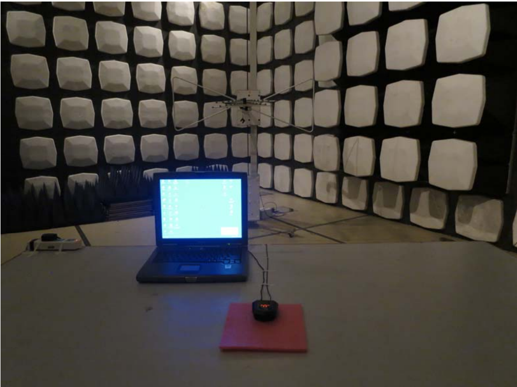
FCC RADIATED EMISSION TEST SETUP
