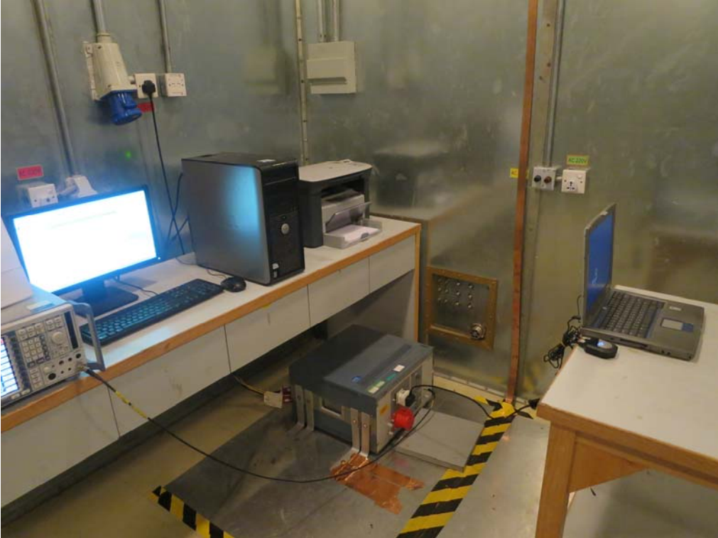
FCC RADIATED EMISSION TEST SETUP
