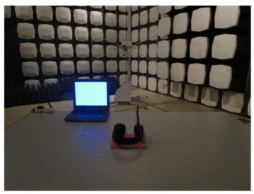
FCC RADIATED EMISSION TEST SETUP
