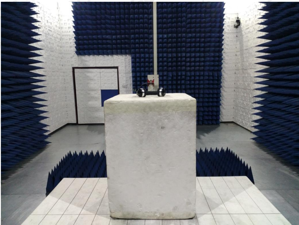
RADIATED EMISSION TEST SETUP ABOVE 1GHZ
