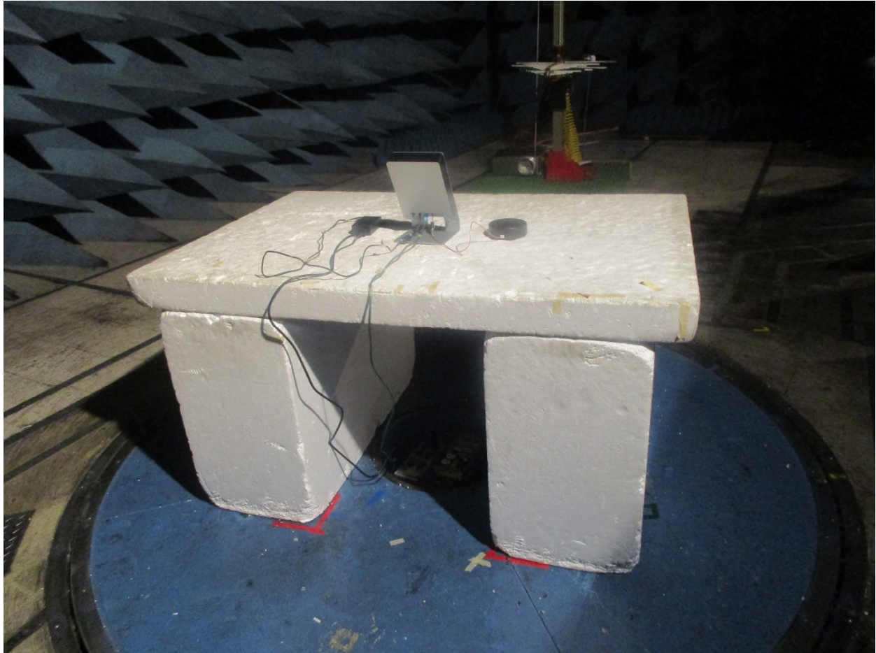
Figure 4: Radiated Emissions – 200 MHz – 1 GHz – Rear View
