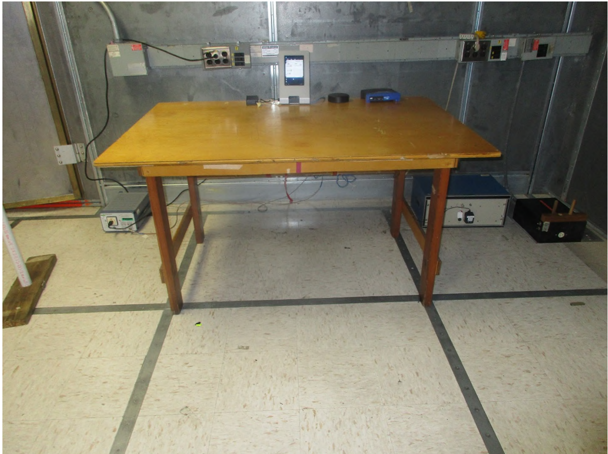
Figure 8: Conducted Emissions – Side View
