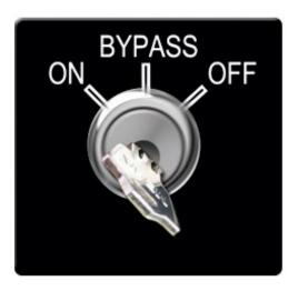
The 'Bypass' mode of operation: When the key switch is turned to the 'Bypass' position, the machine functions just like any other soda dispensing machine. It bypasses all of the ValidFill components. This function is set up as a backup in case a component stops working. It can also be used to allow free soda dispensing.
