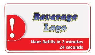
This error message appears when a user tries to refill his or her cup too quickly after the previous fill. The Validfill system is set up so that a user can only refill their cup once per given unit of time (the standard is 5 minutes).
