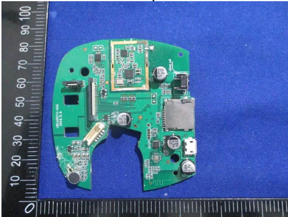
EUT – Main Board Top Unshielded View
