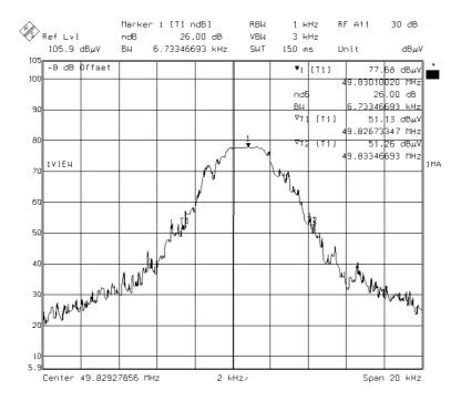
Note: The point T1 (49.826 MHZ) is 26dB below the carrier and inside the operation band 49.82 – 49.90 MHz. This device does meet the FCC requirement.
