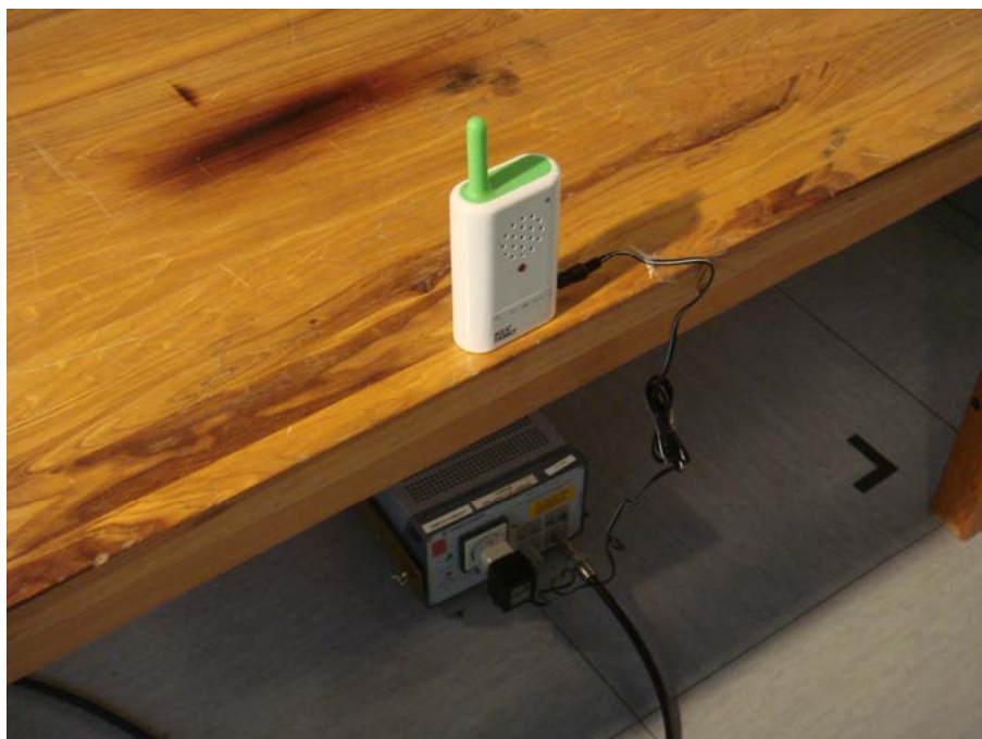
Conducted emission Test setup Photo
