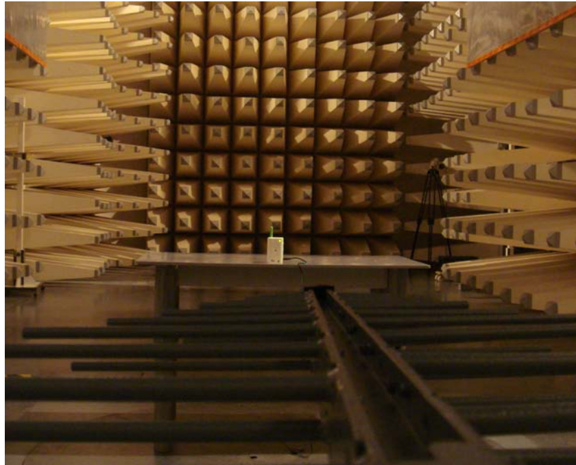
Radiated emission Test setup Photo
