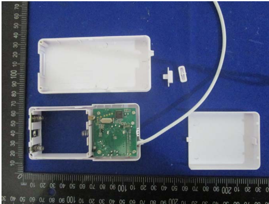
EUT – Transmit Unit Uncover View
