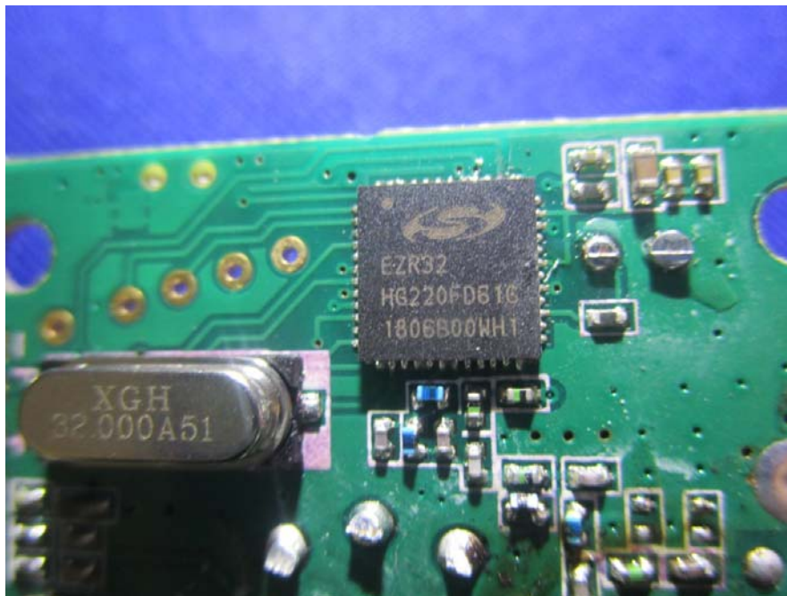
EUT – Transmit Unit Main Chip View
