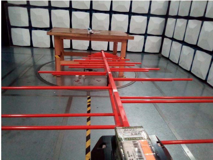
Radiated Emission View (Below 1GHz)
