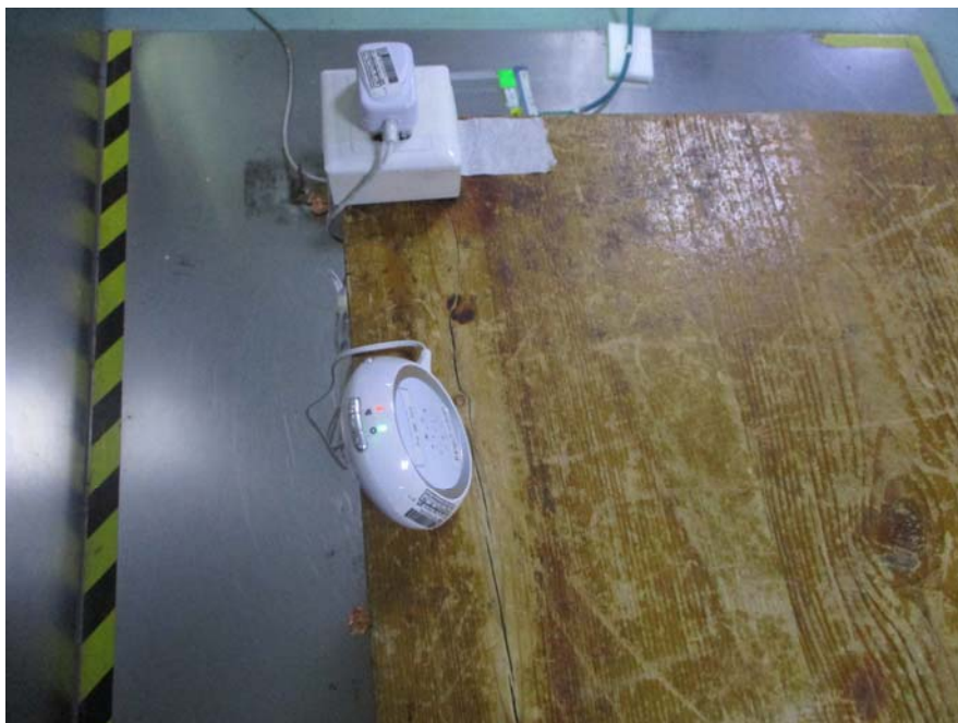
Conducted Emissions – Side View
