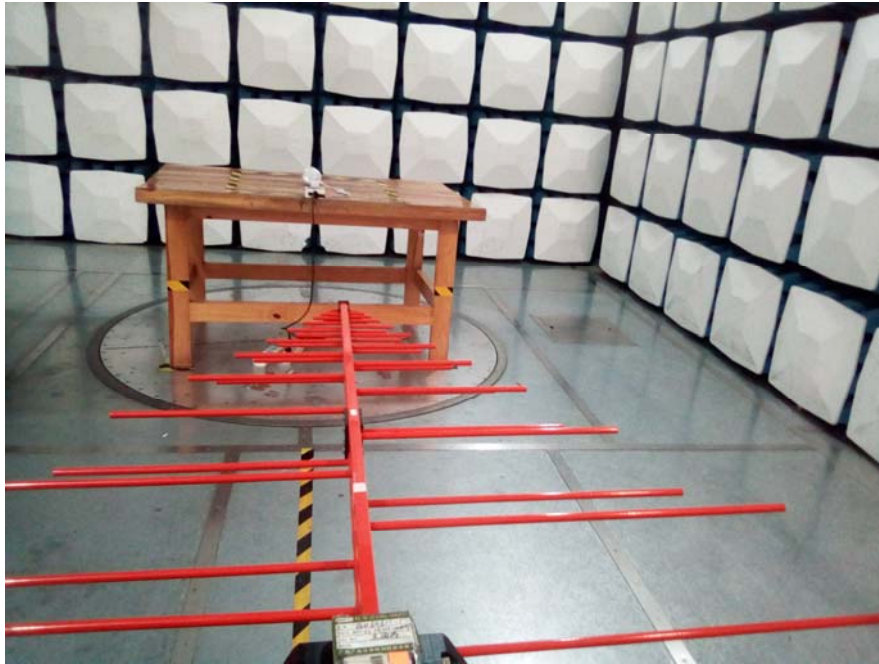
Radiated Emission View (Below 1GHz)
