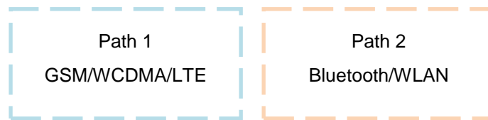
Fig.15.1 Simultaneous Transmission Paths
