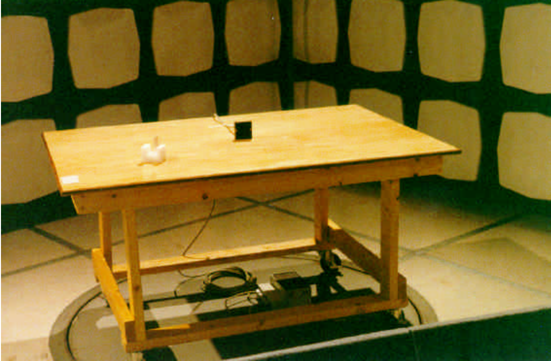
Test Setup in Semianechoic Chamber. Cable was re-wrapped non-inductively during the test. (See report for details.)
