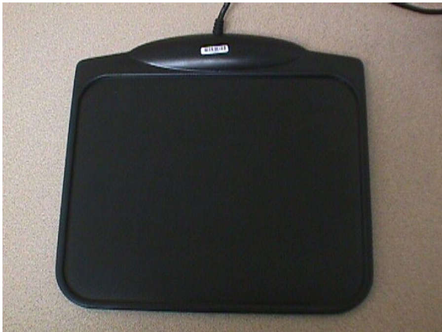
FIGURE 8: Mousepad Plastic Housing Inside Top Half Top Side Without Mat
