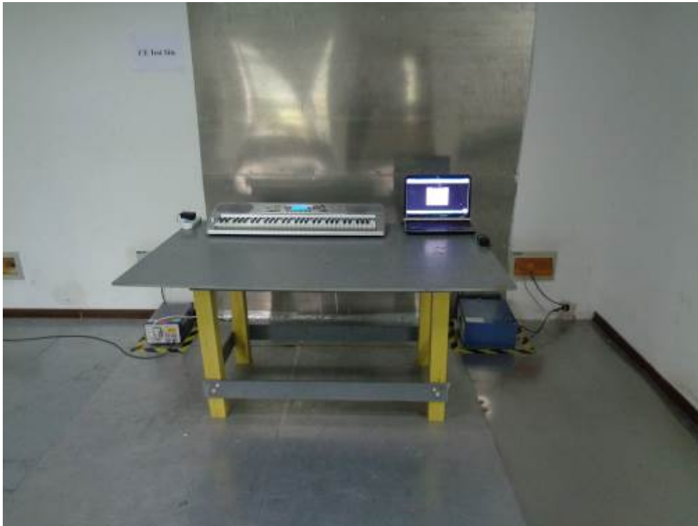
Conducted Emissions Test Setup Front View
