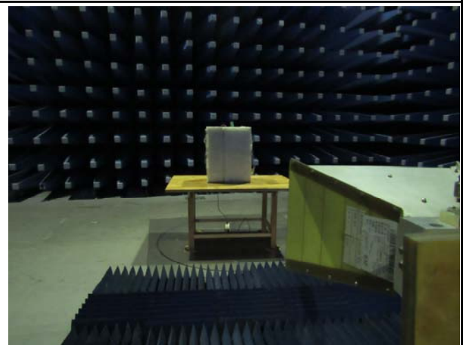
Radiated Spurious Emissions Test Setup Above 1GHz
