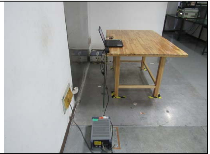
Conducted Emissions Test Setup Side View
