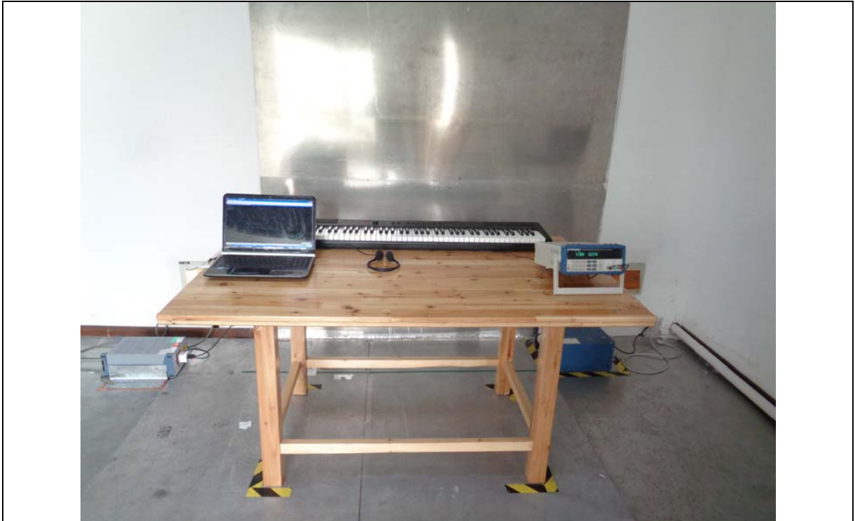
Conducted Emissions Setup Front View
