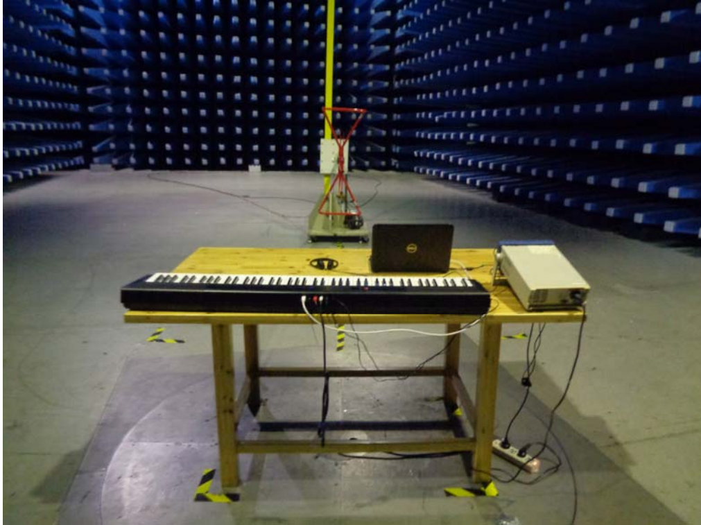
Radiated Emissions Setup Below 1GHz Front View
