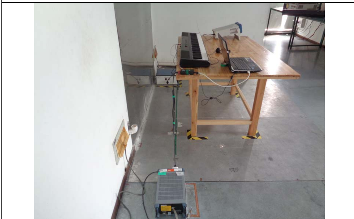
Conducted Emissions Setup Side View
