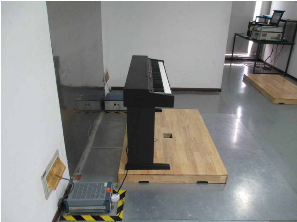
Conducted Emissions Setup Side View
