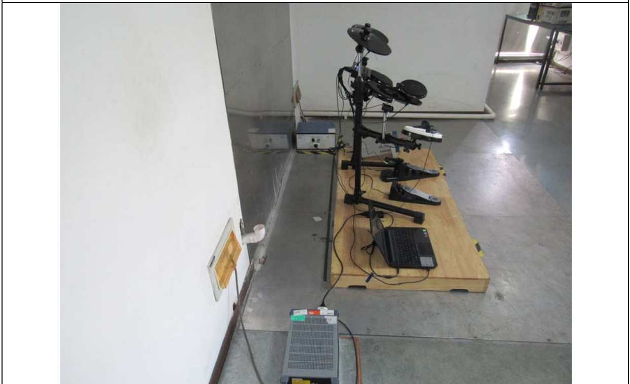
Conducted Emissions Setup Side View
