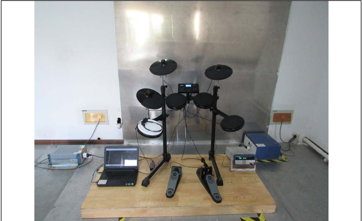
Conducted Emissions Setup Front View
