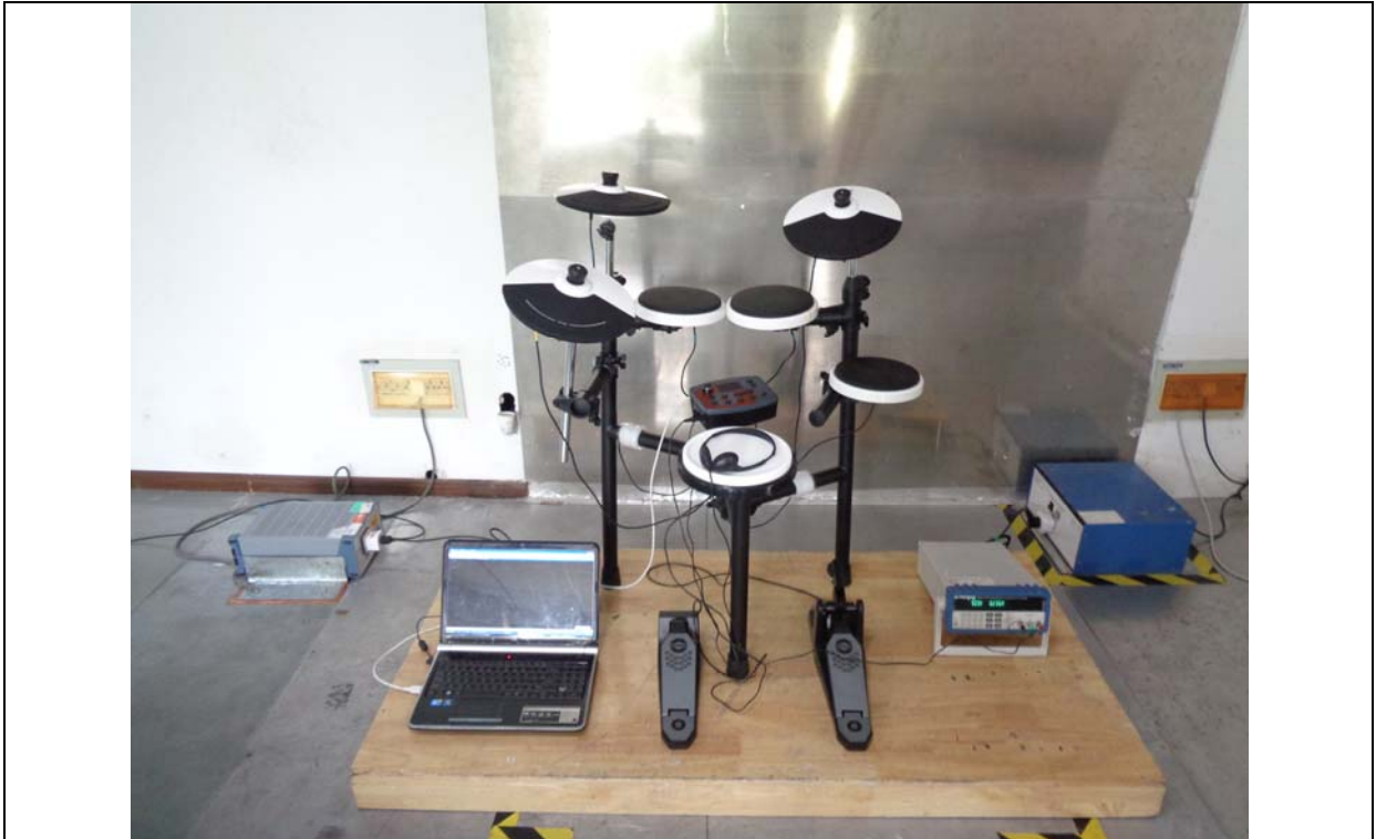
Conducted Emissions Setup Front View
