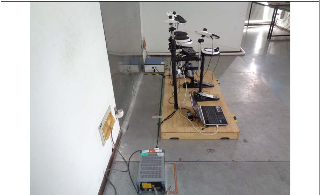
Conducted Emissions Setup Side View
