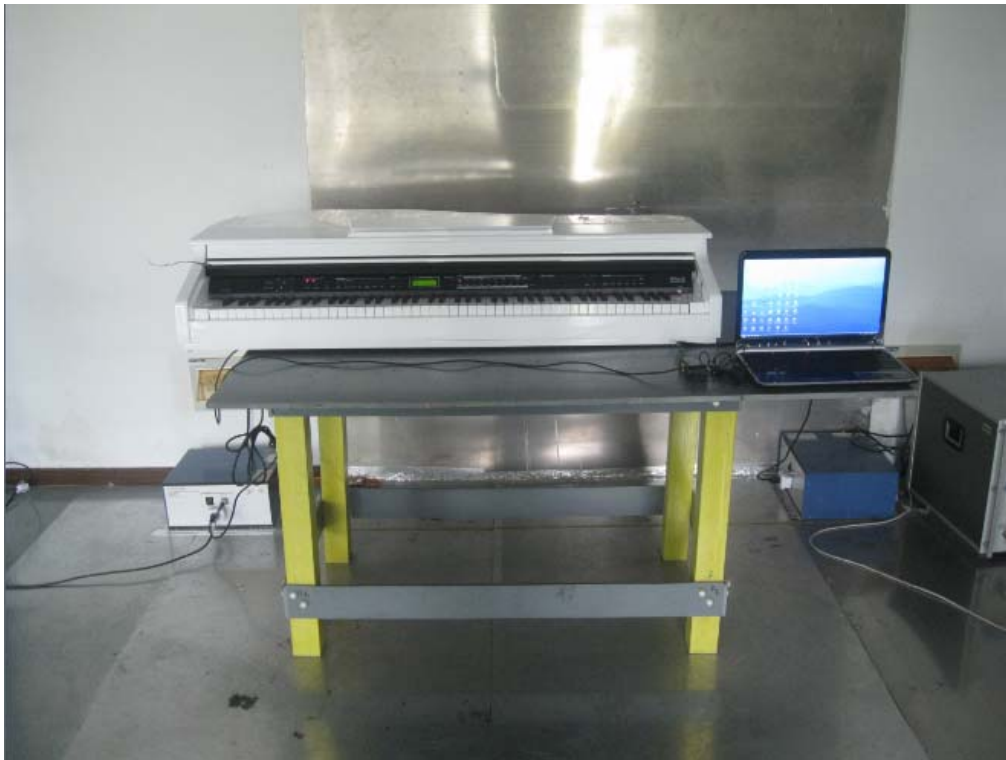
Conducted Emissions Test Setup - Front View
