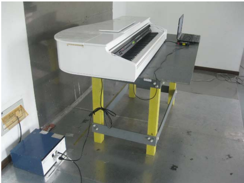
Conducted Emissions Test Setup - Side View
