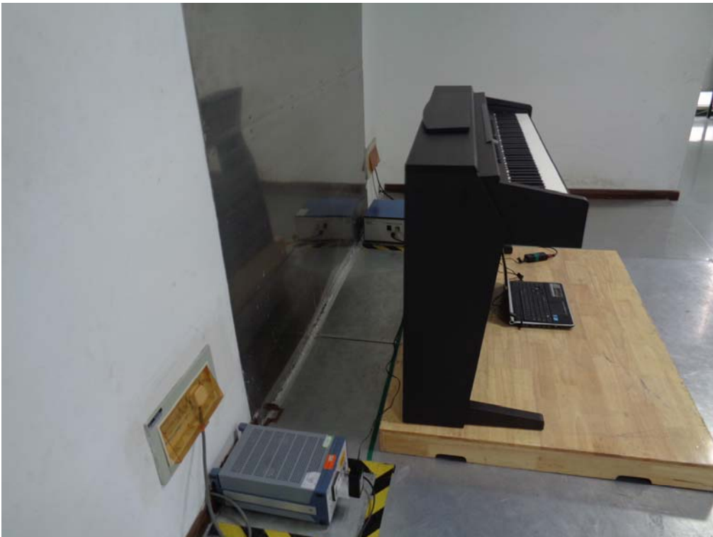
Conducted Emissions Setup Side View
