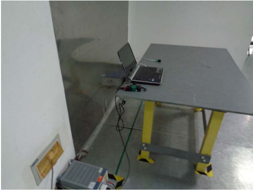
Conducted Emissions Test Setup Side View
