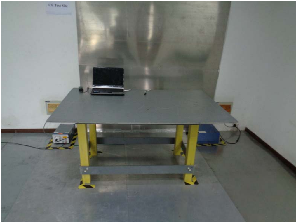
Conducted Emissions Test Setup Front View
