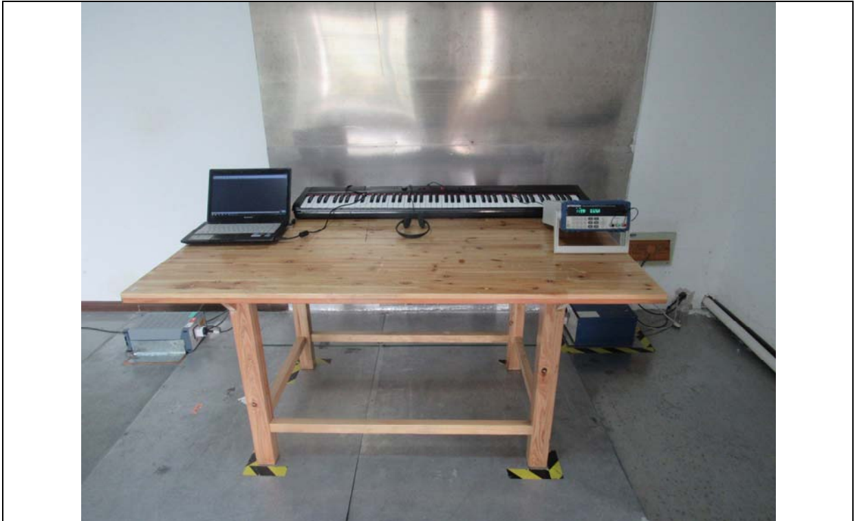
Conducted Emissions Setup Front View
