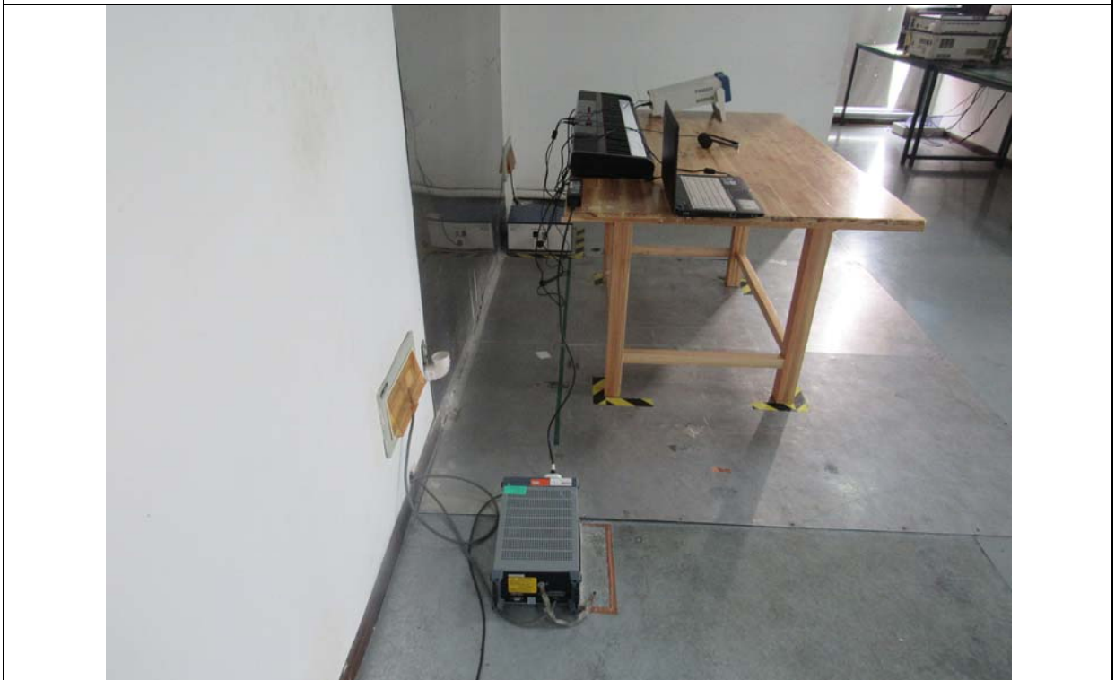
Conducted Emissions Setup Side View
