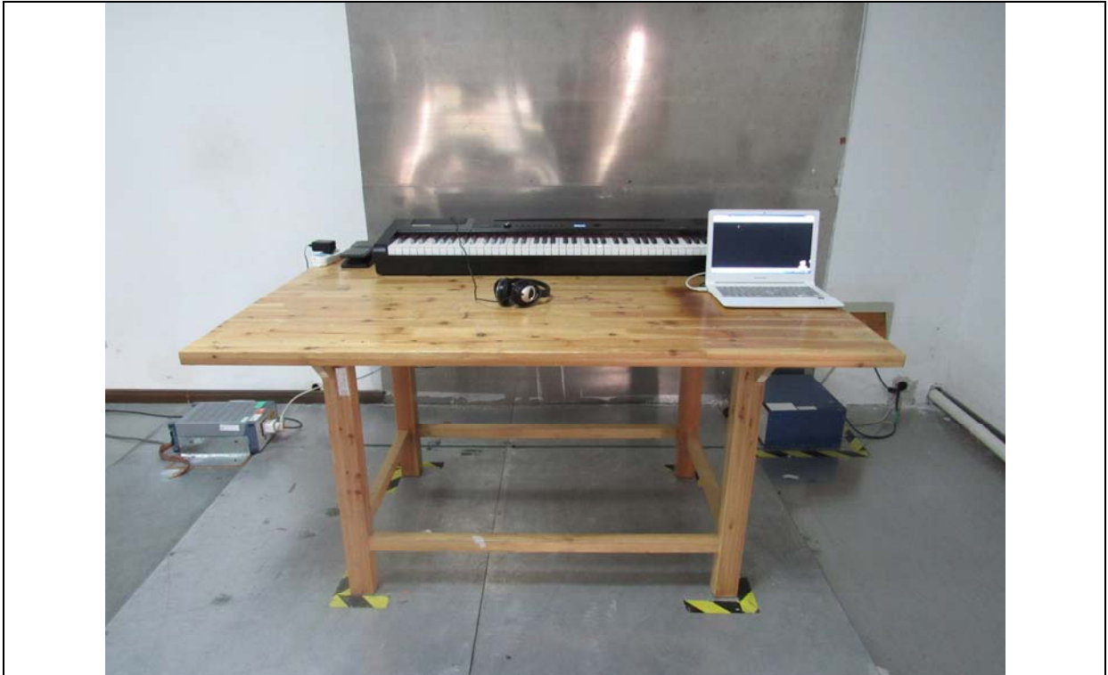
Conducted Emissions Setup Front View
