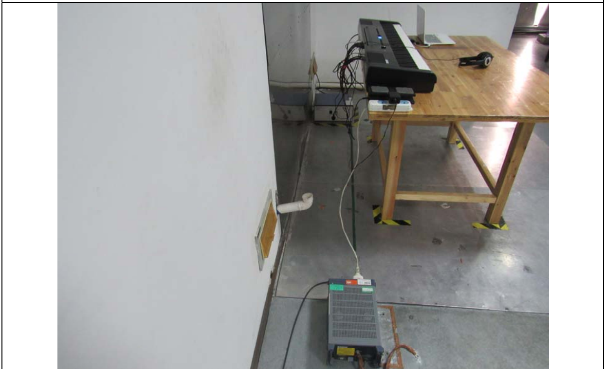
Conducted Emissions Setup Side View
