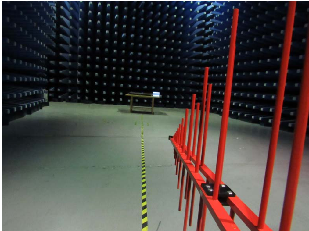
Radiated Emissions Setup Below 1GHz Front View
