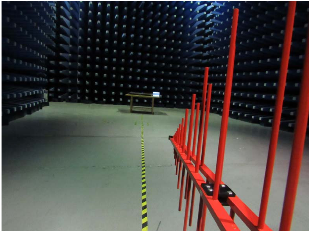
Radiated Emissions Setup Below 1GHz Front View
