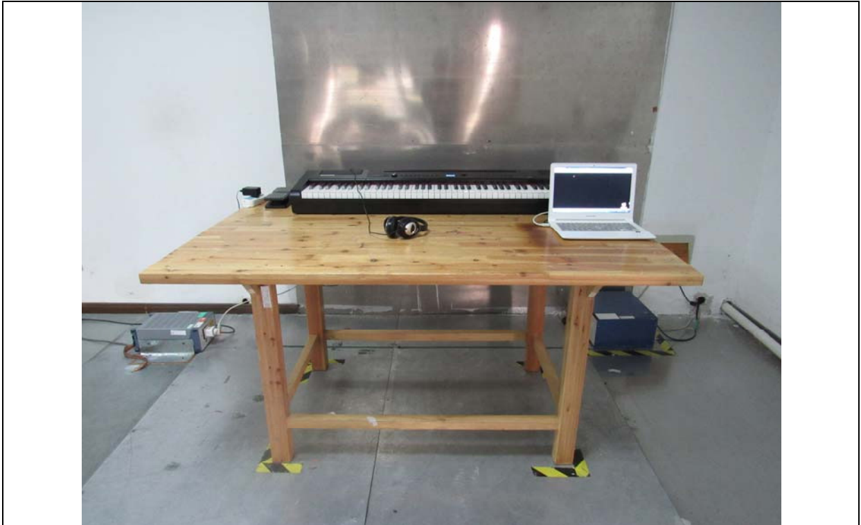
Conducted Emissions Setup Front View
