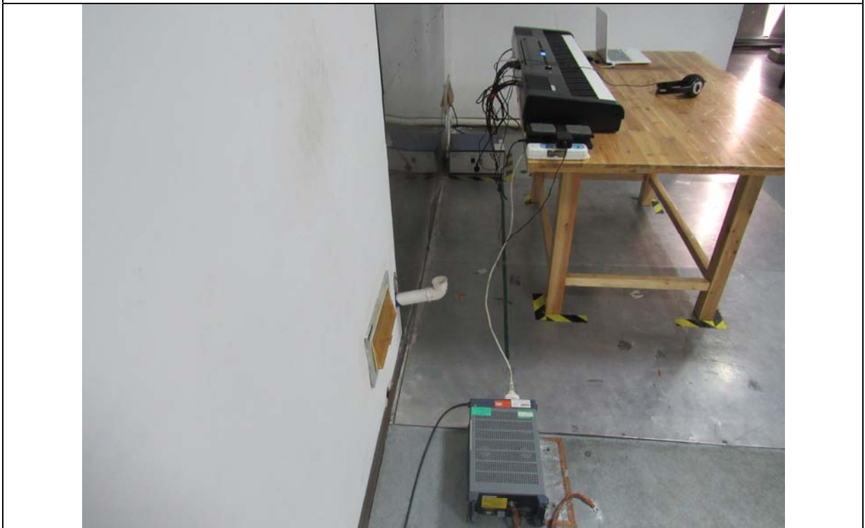
Conducted Emissions Setup Side View
