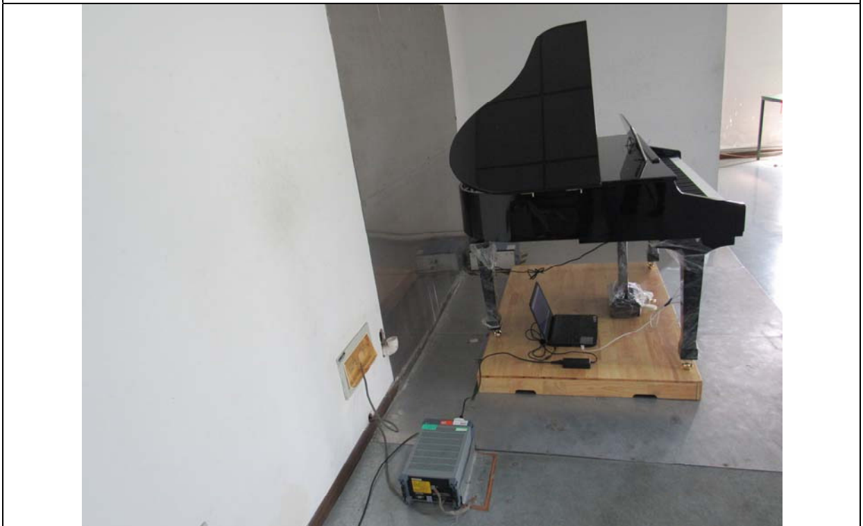
Conducted Emissions Setup Side View
