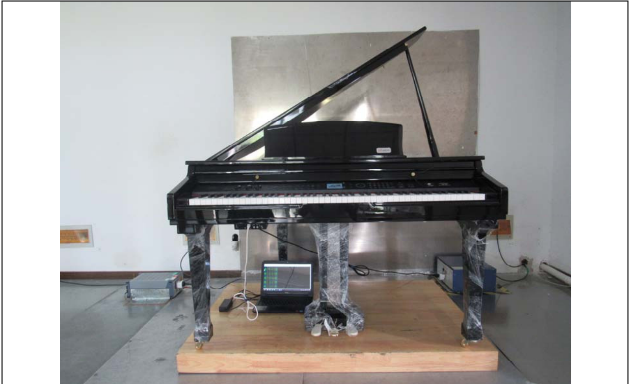
Conducted Emissions Setup Front View
