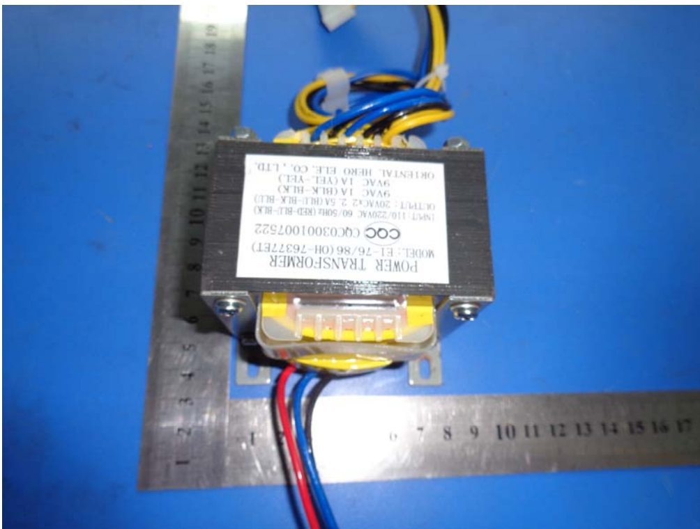
EUT POWER TRANSFORMER– Front View
