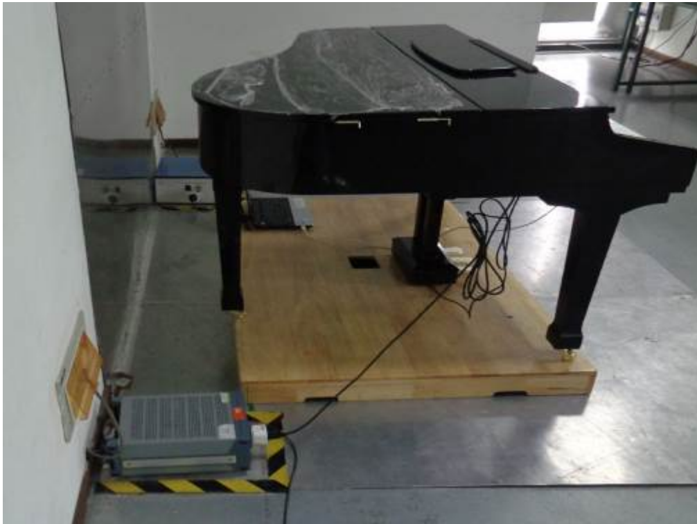
Conducted Emissions Setup Side View
