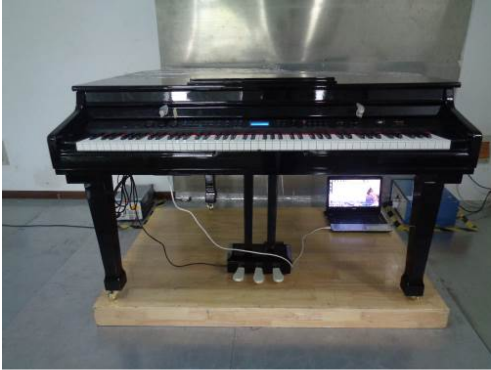
Conducted Emissions Setup Front View
