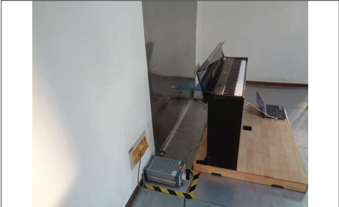
Conducted Emissions Setup Side View
