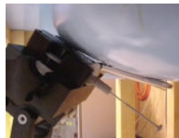
Figure 9. Head SAR Test Setup
