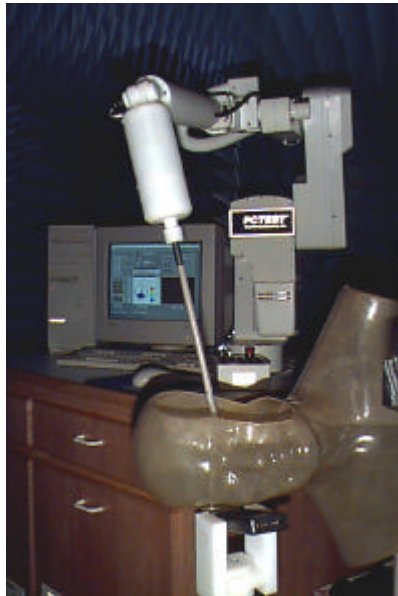
Figure 5. Photograph of the Probe and the Phantom
