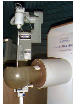
Figure 1. SAR Test Set-up
