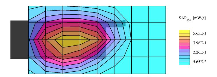
Generic Twin Phantom; Flat Section; Position: (270°,270°); Probe: ET3DV6 - SN1387; ConvF(6.43,6.43,6.43); Crest factor: 1.0; Muscle 835 MHz:  $\sigma=0.95$  mho/m  $\epsilon_r=56.1~\rho=1.00~g/cm^3$  Coarse: Dx=20.0,~Dy=20.0,~Dz=10.0
