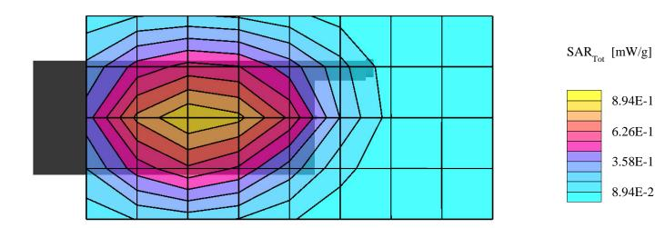
Generic Twin Phantom; Flat Section; Position: (270°,270°); Probe: ET3DV6 - SN1387; ConvF(6.43,6.43,6.43); Crest factor: 1.0; Muscle 835 MHz:  $\sigma=0.95$  mho/m  $\epsilon_r=56.1$   $\rho=1.00$  g/cm³ Coarse: Dx = 20.0, Dy = 20.0, Dz = 10.0
