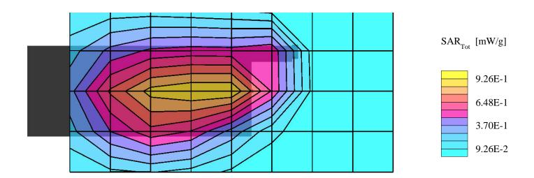
Generic Twin Phantom; Flat Section; Position: (270°,270°); Probe: ET3DV6 - SN1387; ConvF(6.43,6.43,6.43); Crest factor: 1.0; Muscle 835 MHz:  $\sigma=0.95$  mho/m  $\epsilon_r=56.1~\rho=1.00~g/cm^3$  Coarse: Dx=20.0,~Dy=20.0,~Dz=10.0
