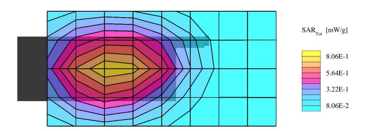
Generic Twin Phantom; Flat Section; Position:  $(270^{\circ},270^{\circ})$ ; Probe: ET3DV6 - SN1387; ConvF(6.43,6.43,6.43); Crest factor: 1.0; Muscle 835 MHz:  $\sigma = 0.95$  mho/m  $\epsilon_r = 56.1$   $\rho = 1.00$  g/cm<sup>3</sup>
