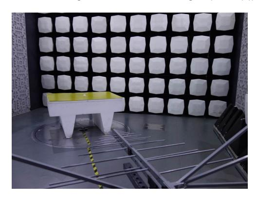
1.1 Radiated Emissions Test Setup
