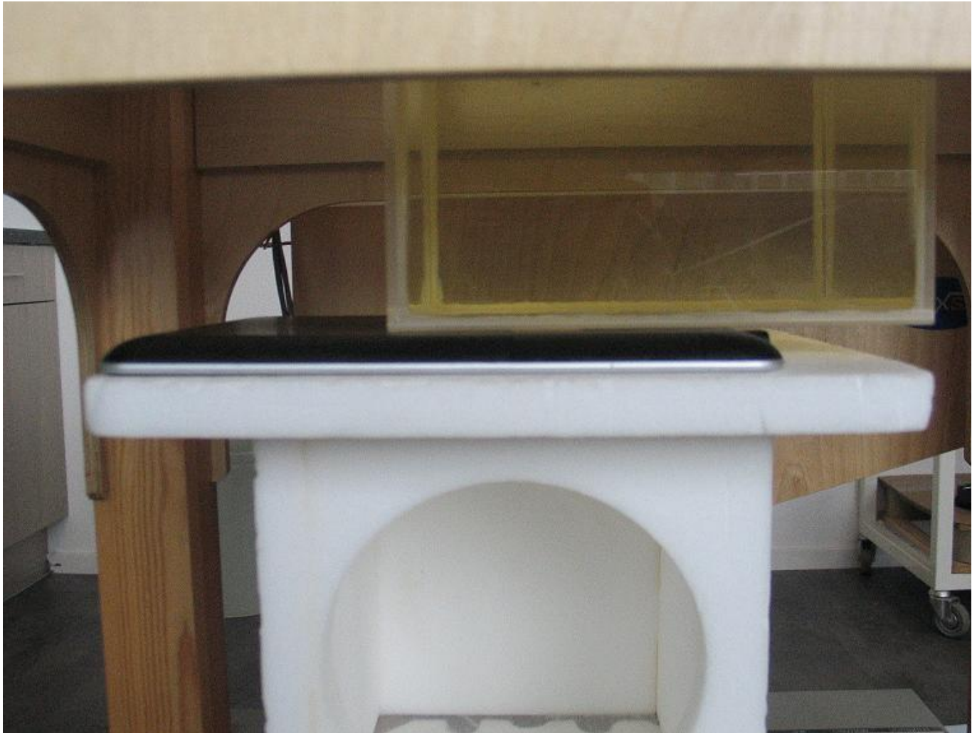
Figure 2: Test setup Bottom measurement (distance EUT-phantom = 0mm).
