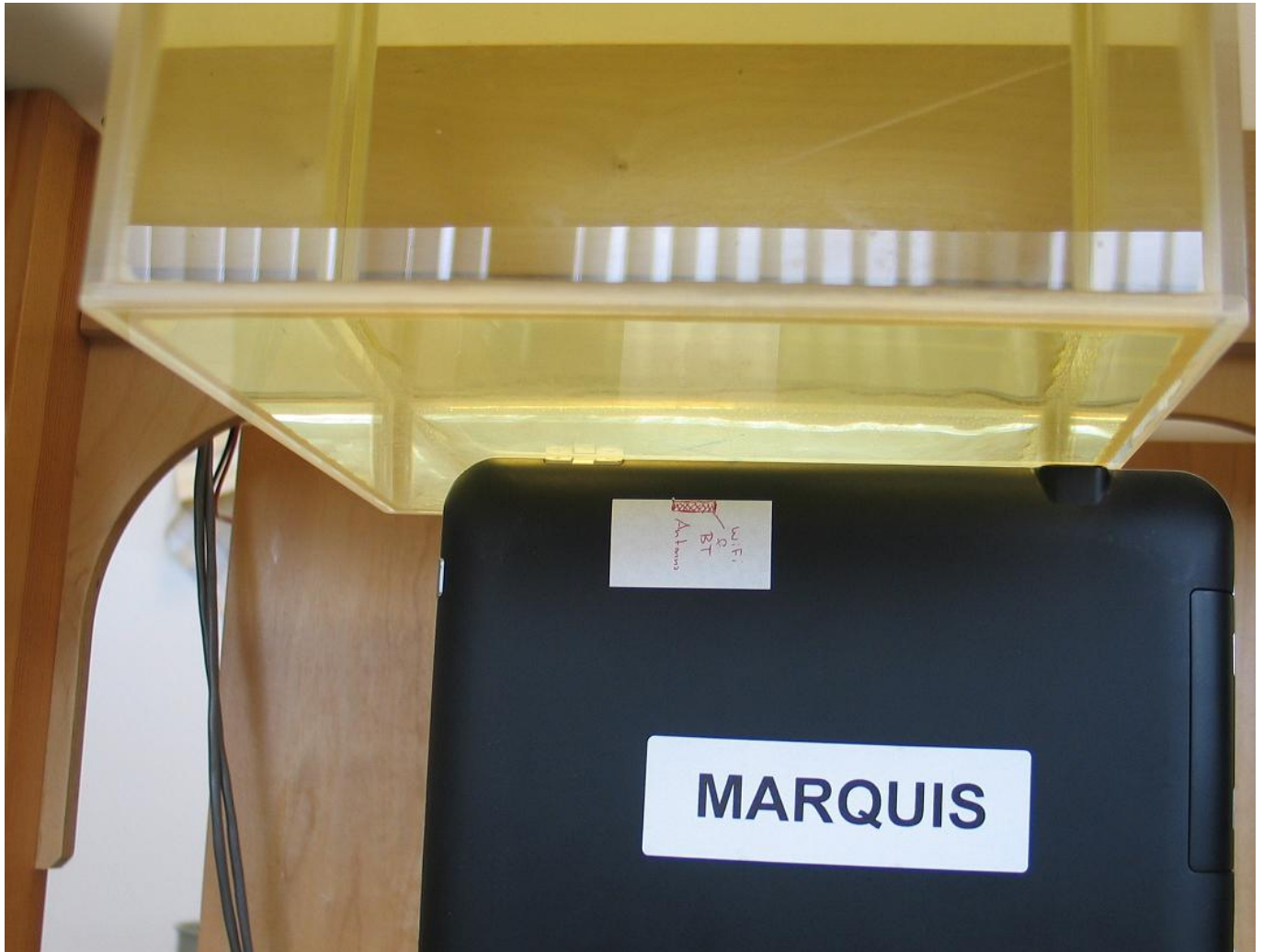
Figure 3: Test setup Edge1 measurement (distance antenna phantom = 10mm).
