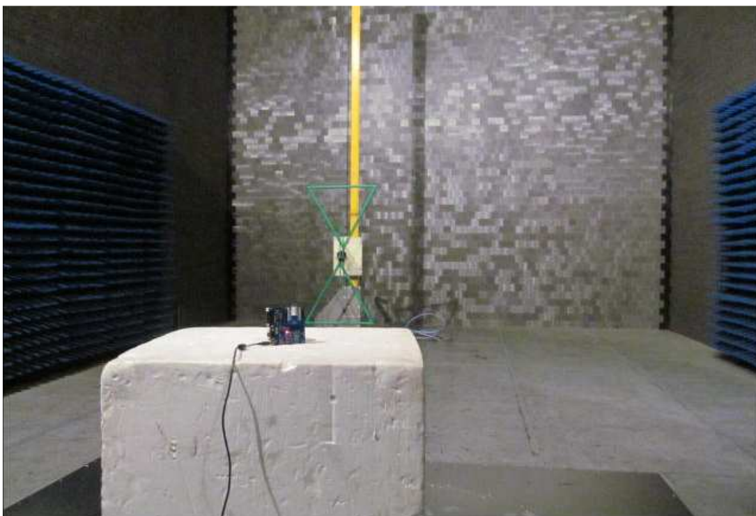
Photograph 2: Set-up for Radiated Emission, 30MHz-1000MHz
