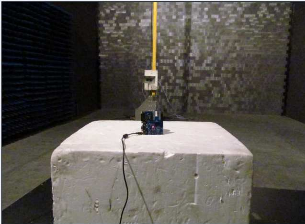
Photograph 3: Set-up for Radiated Emission, 1G-18GHz
