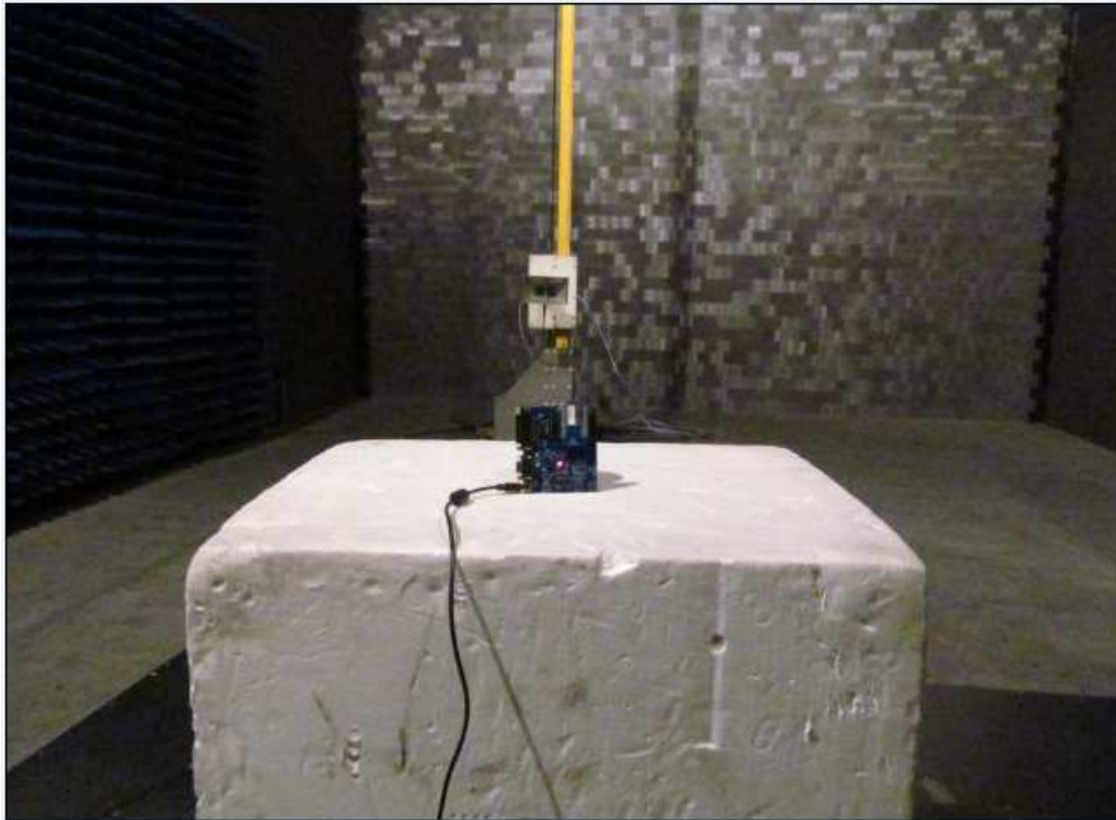
Photograph 3: Set-up for Radiated Emission, 1G-18GHz
