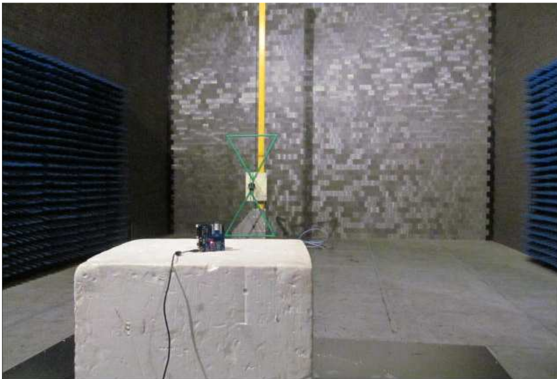
Photograph 2: Set-up for Radiated Emission, 30MHz-1000MHz
