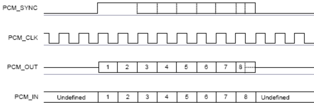
Figure 5: Long Frame Sync (Shown with 8-bit Companded Sample)
