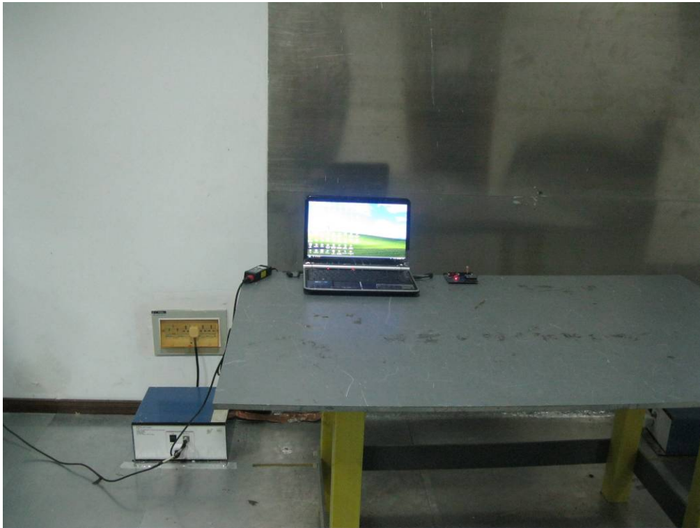
Conducted Emissions Test Setup - Front View
