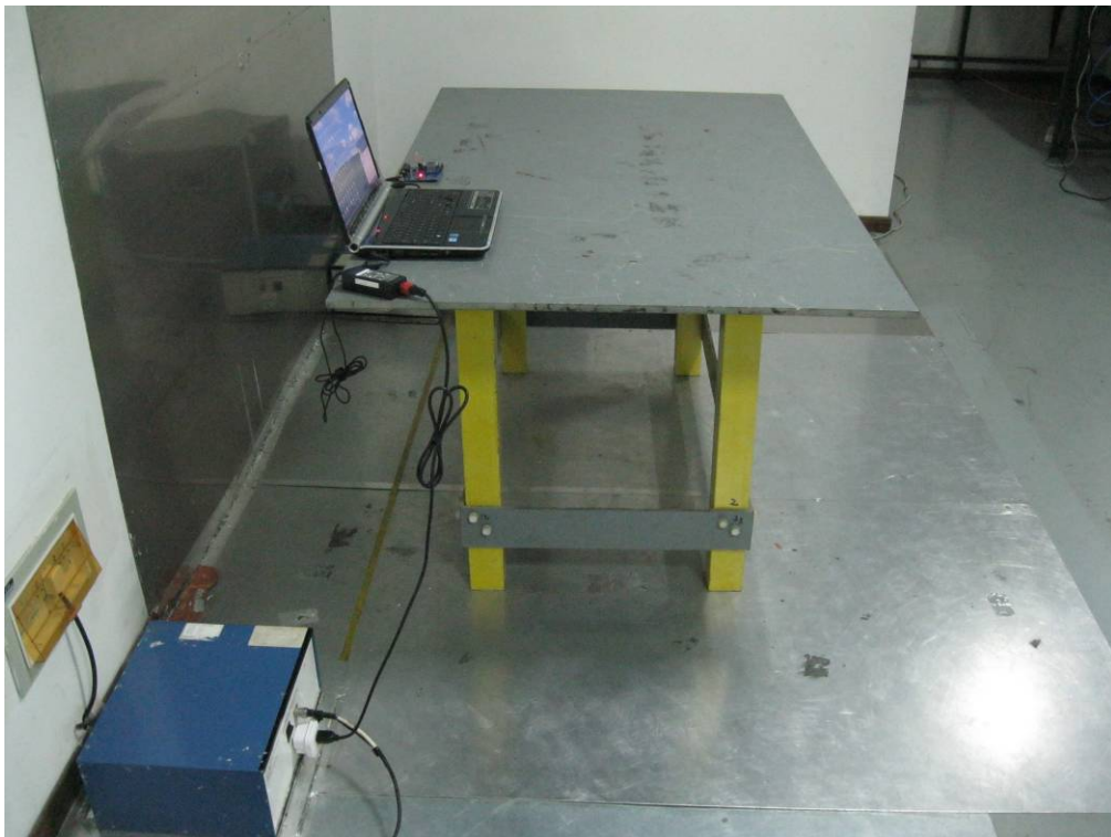
Conducted Emissions Test Setup - Side View
