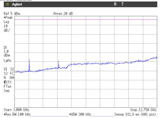
Note: The limit shown in the plot is extrapolated for 100 kHz measurement bandwidth.
