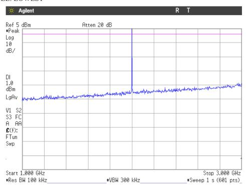
Note: The peak above the limit is the carrier frequency. The limit shown in the plot is extrapolated for 100 kHz measurement bandwidth.
