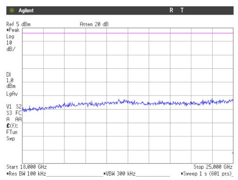
Note: The limit shown in the plot is extrapolated for 100 kHz measurement bandwidth. (This plot is valid for all three channels).
