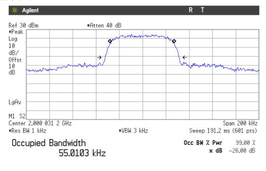
Transmit Freq Error -430.242 Hz x dB Bandwidth 63.390 kHz
