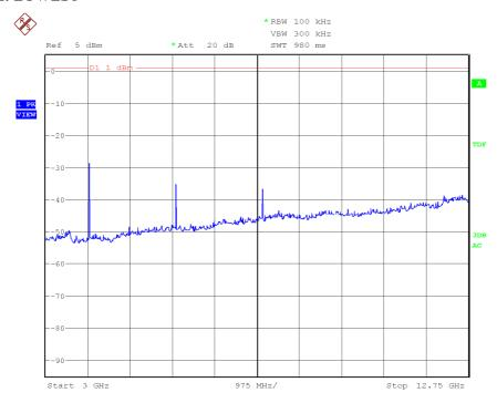
Note: The limit shown in the plot is extrapolated for 100 kHz measurement bandwidth.
