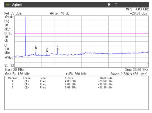
Note: The peak above the limit is the carrier frequency. The limit shown in the plot is extrapolated for 100 kHz measurement bandwidth.
