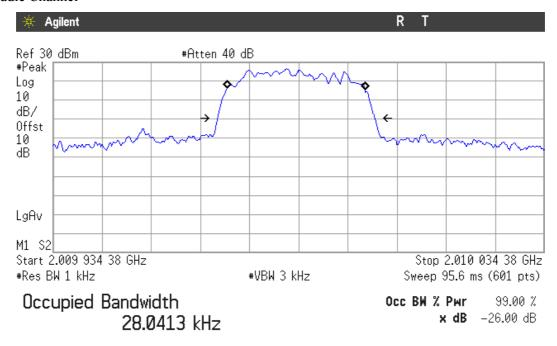
Transmit Freq Error -577.295 Hz x dB Bandwidth 31.956 kHz
