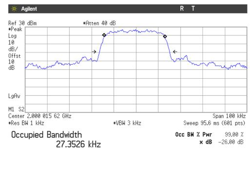
Transmit Freq Error -698.452 Hz x dB Bandwidth 31.526 kHz
