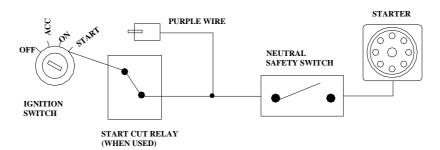
Careful consideration for the connection of this wire must be made to prevent the vehicle from the starting while in gear. Understanding the difference between a mechanical and an electrical Neutral Start Switch will allow you to properly identify the circuit and select the correct installation method. In addition you will realize why the connection of the safety wire is required for all mechanical switch configuration.
