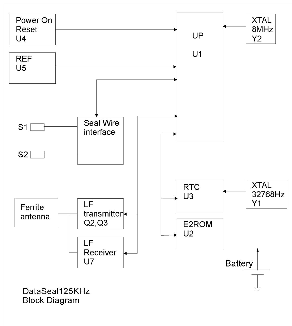
4.2. **μP** (U1 Pg.2): PIC18LC252 μP timed by an 8 MHz ceramic resonator (Y2 Pg.2).
