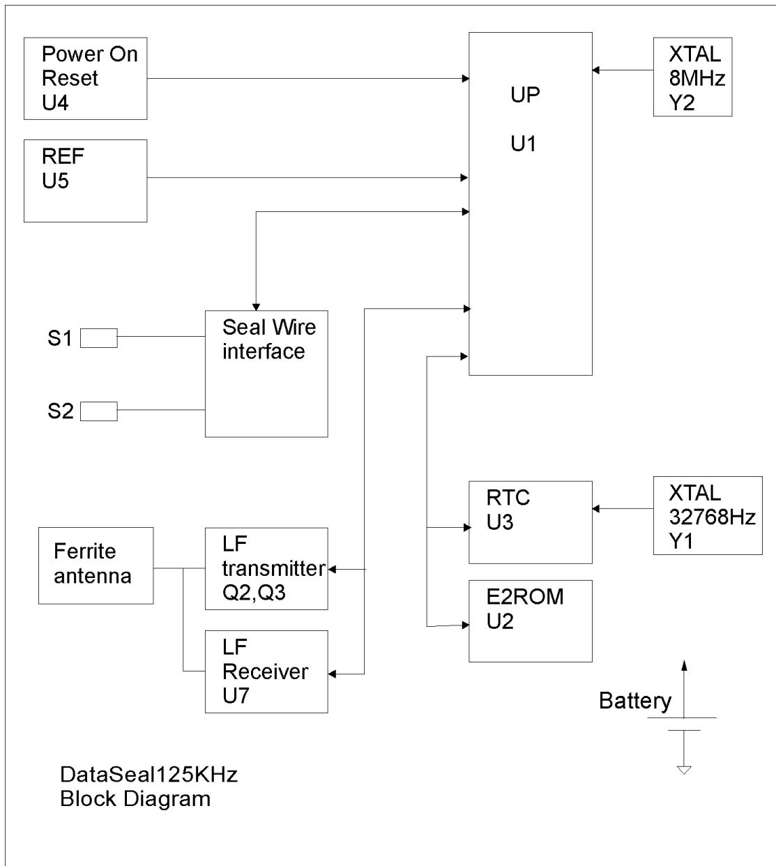
4.2. **IP ( U1 Pg.2 )** : PIC18LC252 IP timed by a 8MHz ceramic resonator (Y2 Pg.2).
