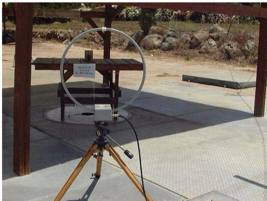
Figure 1. Radiated Emission Test 9kHz-30MHz
