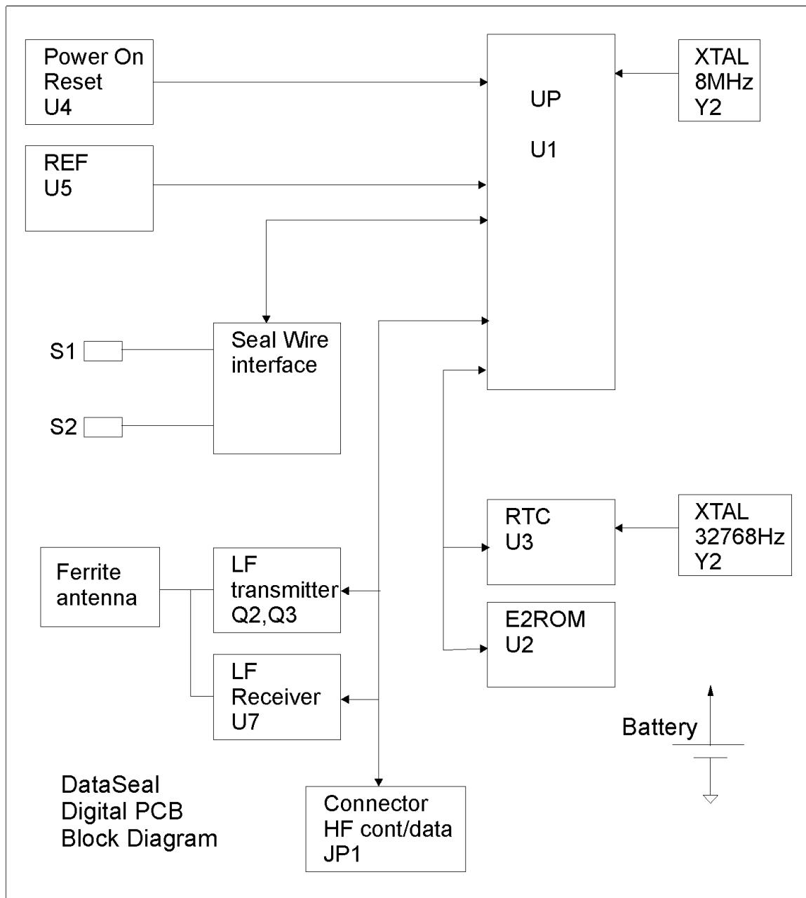
5.2. **μP (U1 Pg.2):** PIC16F876 μP timed by an 8MHz ceramic resonator.
